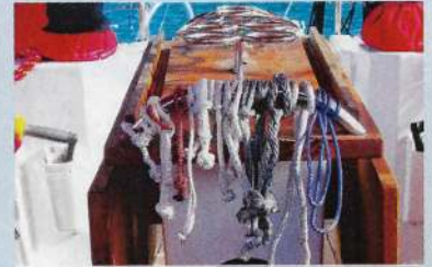
A collection of Dyneema soft shackles and loops is useful to have on board
