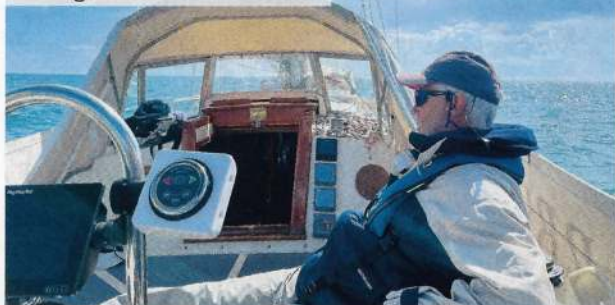
The addition of a bow thruster at the helm has reduced stress during berthing and the need to run around
