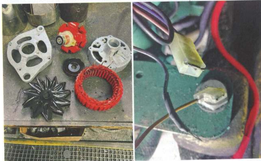
LEFT The alternator's refurbished components RIGHT Spade connector had snapped off
