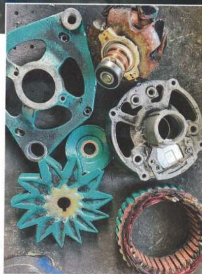
ABOVE Refurbished components reassembled into an alternator RIGHT The old alternator stripped down
