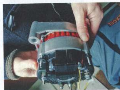
Wiring terminals at the back disappear from view once installed
