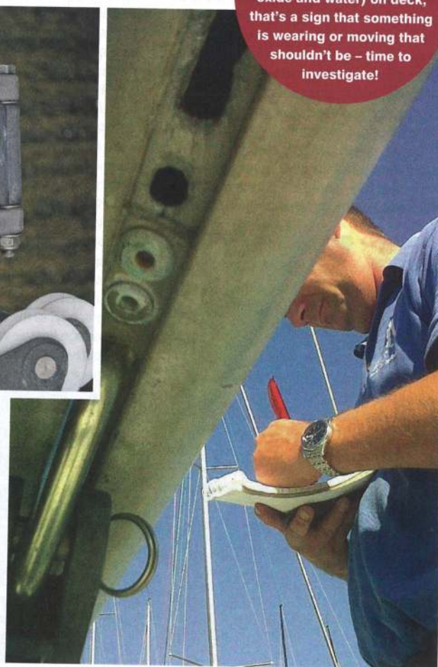
ABOVE Check the boom's fittings for any movement RIGHT A checklist is a good idea to ensure nothing gets overlooked
