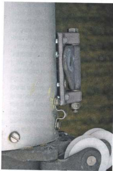
ABOVE Check the boom's fittings for any movement RIGHT A checklist is a good idea to ensure nothing gets overlooked
