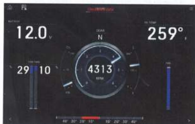
LEFT Newer engines and displays enable a screenshot to be taken of the various engine parameters and are an easy way to store a lot of data. The file name usually has a date on it as well
