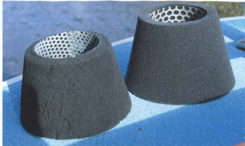
ABOVE The old air filter (left) next to the new filter (right). This may explain the silicon in the oil analysis, as the filter appears not to have been changed for many years
