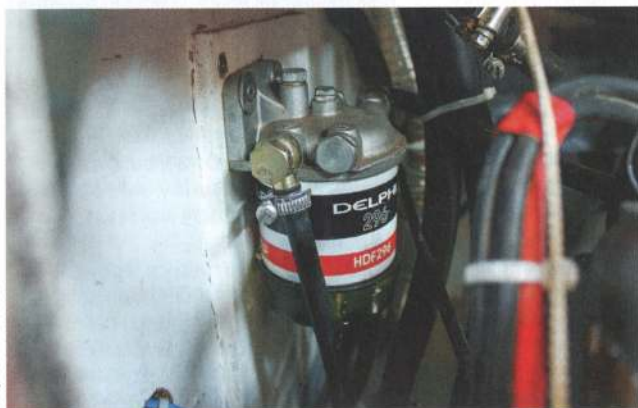
The CAV296 type fuel filter that's typically used for smaller marine diesel engines
