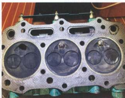
LEFT Geoff's Bavaria 39 Tessa Jane ABOVE RIGHT The precombustion chamber insert on the left cylinder has completely disappeared
