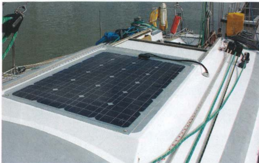
ABOVE A simple solar system with a 60-100W panel on the coachroof can transform the robustness of an electrical system
