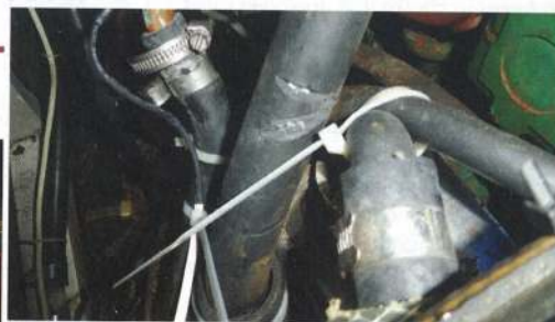
ABOVE A nasty case of cable ties cutting into the outer casing of the header tank feed hose
