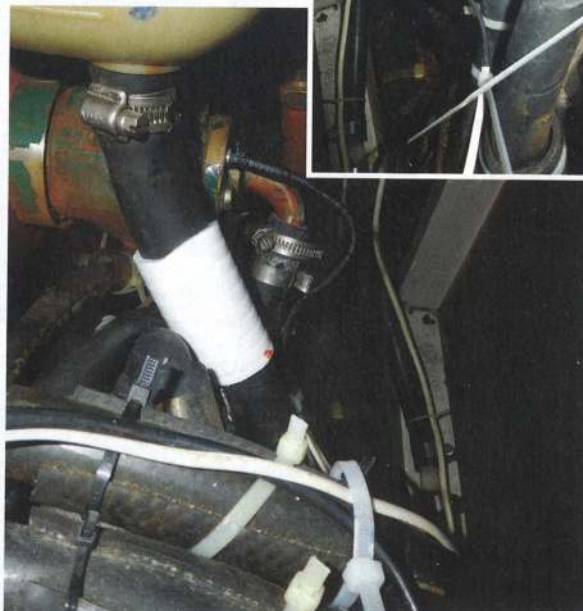
ABOVE A nasty case of cable ties cutting into the outer casing of the header tank feed hose
