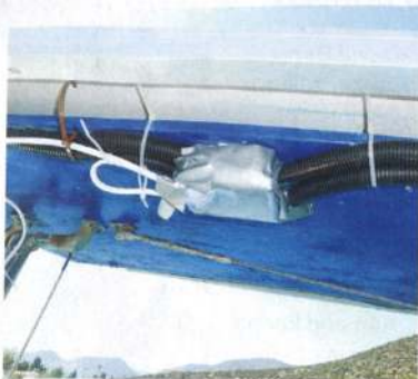
Solar panels get-us-home fix meant running the wire from this box local to the panels to the controller along the outside of the boat...
