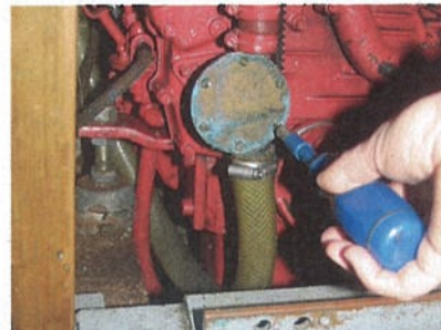
Not every water pump impeller housing is as easy to reach as this one. Removing a damaged impeller can be tricky
