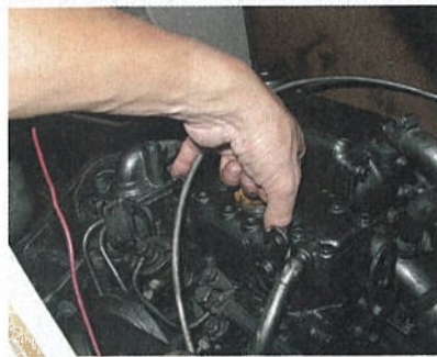
Holding decompression levers open while cranking gives a low battery a better chance of spinning the engine up to speed
