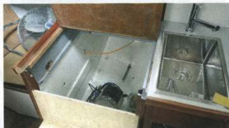
With very few moving parts, an electric motor takes up far less room, though batteries tend to make the overall weight about the same
