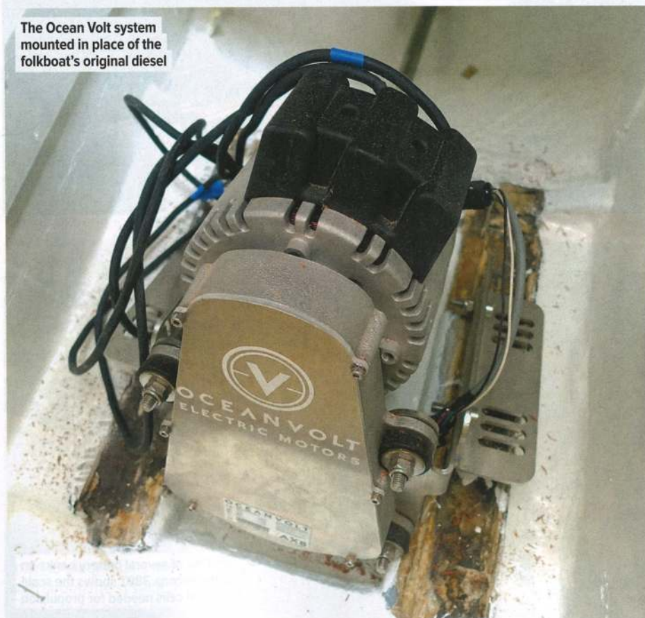
With very few moving parts, an electric motor takes up far less room, though batteries tend to make the overall weight about the same
