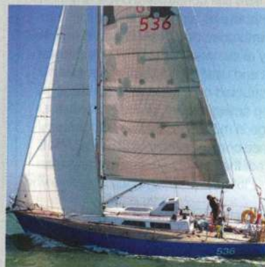
This mainsail has completed 20,000 miles of offshore racing. A two ply leech was fitted when the sail had covered 12,000 miles and extra reinforcement around the first reef leech reinforcing patch after 18,000 miles.
