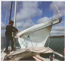
UNDERWAY For ease and safety, have the halyard led back to the cockpit. Once underway, motoring slowly and just off the wind about 10°, undo the sail ties as you walk towards the mast. The sail is likely to drop to the leeward side as it falls off the boom. With halyard winches at the mast, if the halyard exit is on the port side, keep the wind on the port bow so you're slightly on the high side and away from the falling sail.
