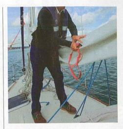
FLAKE THE SAIL With no lazyjacks, flake sail over the boom if possible or put the sail on top of the boom as tidily as you can, and secure with sail ties. Tie them in the same direction and on the same side as the halyard exit at the mast, as it makes it much easier to undo them as you walk towards the mast from the cockpit.
