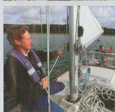
EASE VANG AND MAINSHEET Next, ease the vang and mainsheet then raise the boom with the topping lift as this takes pressure out of the sail, which makes reefing easier.
