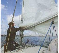
The task now is to hoist as quickly as possible. Having the boom raised means the sail cannot power up during the hoist. The last part of the hoist is always harder as there is more sail aloft, more of the sail is being caught by the wind and your arms are gradually becoming tired. Be sure to keep control of the reefing lines to prevent them wrapping around the topping lift.
