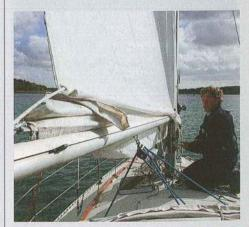
SET THE SAIL AND TRIM With the cringle pulled right down to the boom, ease the topping lift, or crank on the vang if you have a rod kicker, to lower the boom and trim the sail. Tidy-up and settle down.
