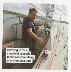
Tacking can be done with ease singlehanded as we only have one sail to worry about; the mainsail will look after itself. After checking to make sure there are no boats close by, we can turn the boat through the wind and effectively heave to, giving us time to ease the old sheet and haul in the new. This will prevent any flogging of the headsail.
