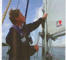
TRIM THE SAIL Once you're happy with the halyard tension, return to the cockpit to ease the topping lift and lower the boom with the vang. You can now trim the sail. Tidy up the reefing lines and halyard tail so that they're ready for use and won't get tangled or go overboard. Then get sailing!
