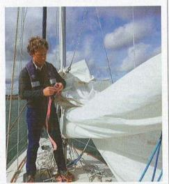
LOWER Lower the mainsail, trying to flake the luff as the sail comes down. When it's lowered, loop the halyard under a winch on the mast and haul the halyard by hand to make fast. This stops the wind hoisting the sail again. Lazyjacks help as they guide the lowering sail on to the boom, which means you don't need to climb on top of anything to secure the mainsail.
