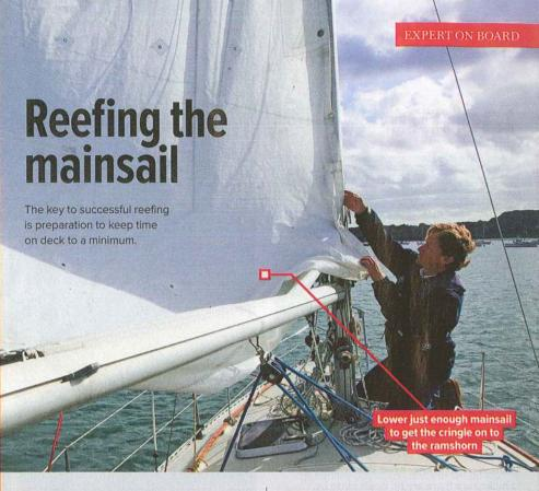
FLAKE THE MAINSAIL HALYARD Make sure the main halyard is flaked out as this will need to run free to lower the mainsail. The new reefing line needs to be around a winch ready to be hauled in.
