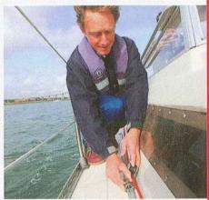
CHECK THE SHEETS Have a guick check of the sheet bowlines on the clew of the sail, the car positions (particularly if you are reefing) and the stopper knots in the ends of the sheets, make sure the furling line is clear to run, and that's just about all that is required.
