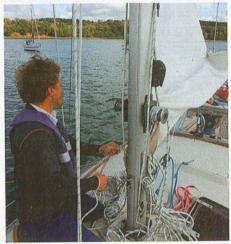
PREPARE TO DROP First, flake the main halyard and grab some sail ties. Next, hoist the boom with the topping lift and make fast. Securing the topping lift is extremely important to prevent the boom from falling down. Now haul on the mainsheet to centre the boom, then turn the boat about 10° off the wind so you stay on the high side and away from falling sail. Now you're ready to drop.
