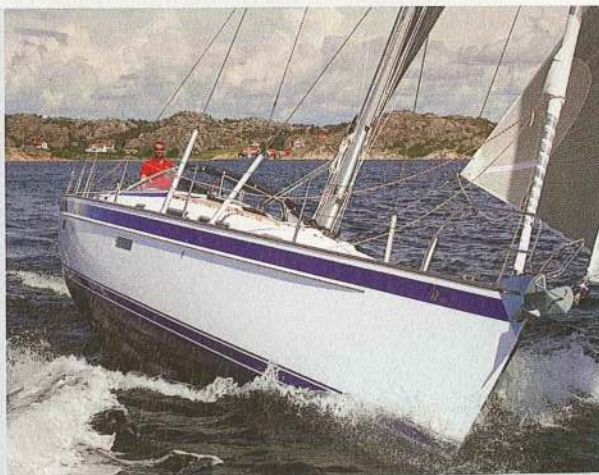
Strakes are evident on this Hallberg-Rassy 412 from Sweden
