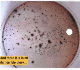
the probability of fuel degradation. There are many contributing factors, including oxidative breakdown from exposure to air and light, hydrolytic breakdown through exposure to water and catalytic breakdown from exposure to certain metals. As far as diesel bug goes, it's the hydrolytic breakdown and build-up of water in the tank that we're really interested in.
