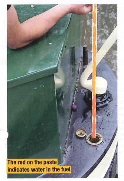
condensation forming on the steel walls of the tank if it's not kept full and some water can even be present in the fuel itself – and how good has the seal been on your filler cap during the winter rains?
