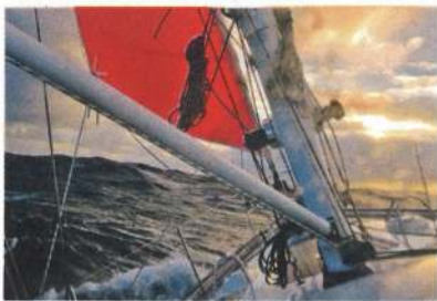
High visibility storm jib set on a yacht on passage from Tasmania to New Zealand
