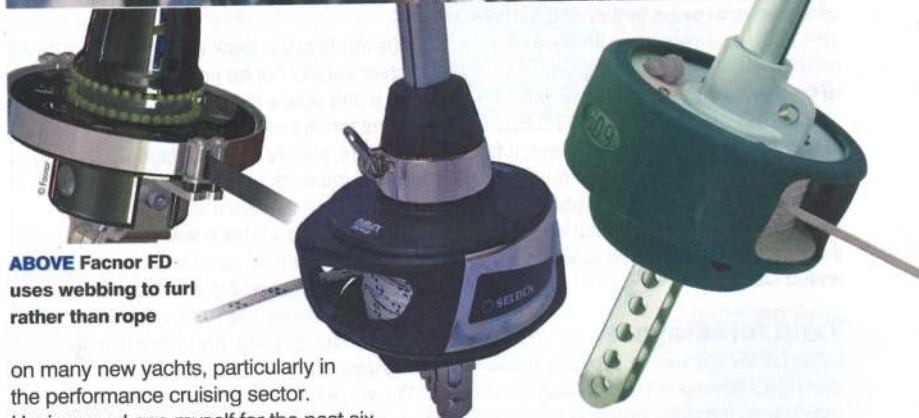
ABOVE Plastimo 609 for boats from 20-30ft ABOVE LEFT Latest generation of Seldén's Furlex 304S for boats up to 15 tonnes displacement
