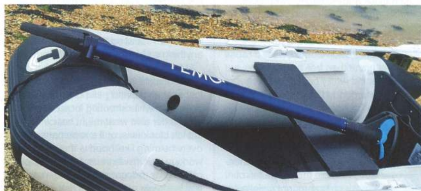
The tiller arm slides into the main body of the outboard making it easy to stow and carry
