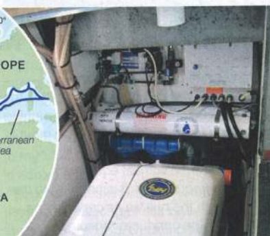
ABOVE LEFT The tubular housings for the watermaker membranes behind the generator's acoustic enclosure. ABOVE RIGHT Our twin boomed headsails which we set for the 18-day easterly trade wind crossing from Sao Vicente in Cape Verde to St Lucia
