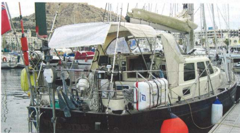
Wild Bird is set up to maintain radio contact. Note the Ampair, towed prop generator, Hydrovane wind-powered steering device and the backstay high frequency (HF) antenna
