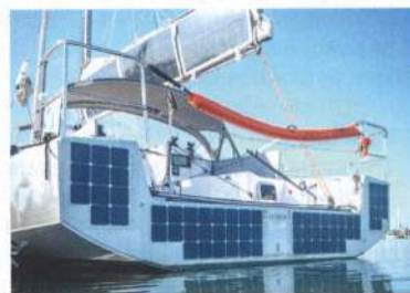
ABOVE LEFT The Raymarine Axiom multi-function display (MFD) has been configured as an energy flow meter RIGHT Transom-mounted solar panels catch reflected sunlight
