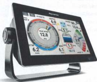
ABOVE LEFT The Raymarine Axiom multi-function display (MFD) has been configured as an energy flow meter RIGHT Transom-mounted solar panels catch reflected sunlight
