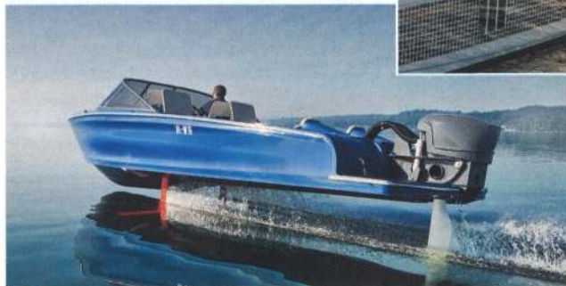
LEFT Grace or pace? The Candela has a top speed of 30 knots thanks to its Torqeedo motor and retractable foils. RIGHT The Spirit 44E is entirely electric. Note the solar panels blended with the lazarette hatch. CENTRE Sunreef 80 Eco, bedecked with 34kW (peak) solar panels
