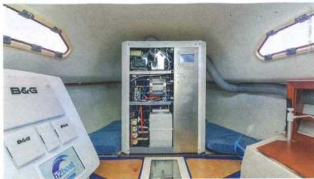
LEFT Italian H2 Boat is trialling a hydrogen fuel cell in a 24ft yacht using a B&G control interface
