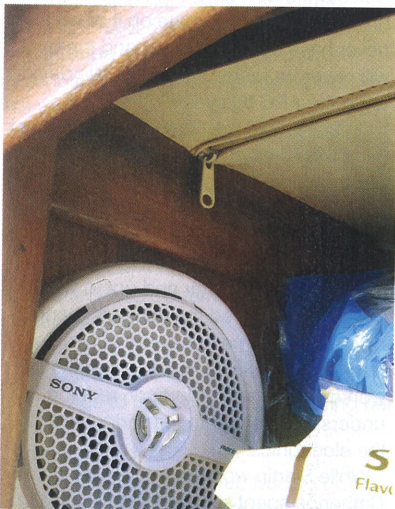
Corroded interior zip on headlining
