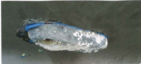
LEFT: A typical hull anode as seen on many boats. Its effectiveness in protecting the propeller is debatable when placed as far forward as this. The white deposits of zinc oxide are inhibiting its action.
