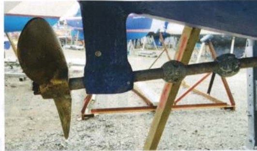
ABOVE: Two anodes have been fitted to this prop shaft to extend life. Ideally they could be closer to the propeller for better protection
