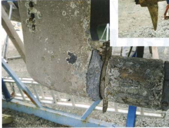
ABOVE: Two anodes have been fitted to this prop shaft to extend life. Ideally they could be closer to the propeller for better protection
