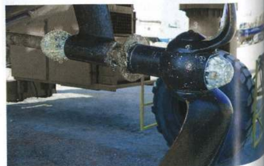
The anode for this feathering prop is small, limiting its life but a shaft anode provides extra protection
