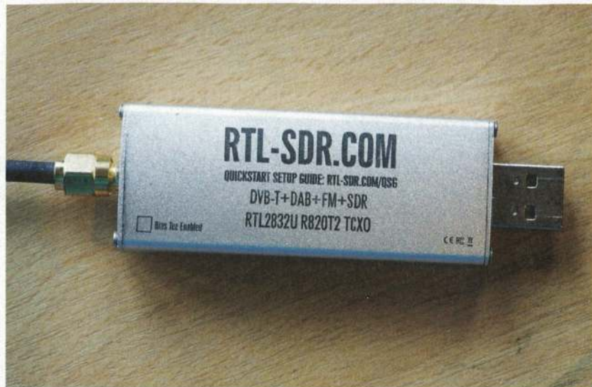
The preferred SDR dongle. Although this cost a little more the circuitry has a guaranteed frequency accuracy that reduces the amount of tweaking necessary to centre on the AIS frequencies
