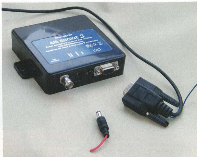
ABOVE NASA Marine's AIS receiver – the 9-pin serial lead on the right has an extra blue flylead which connects to the NMEA output of a GPS receiver. The serial lead then feeds into a laptop
