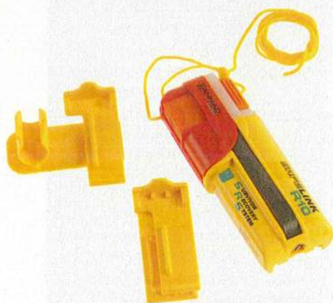
The Kannad SAFELINK R10 SRS AIS MOB can be mounted on a lifejacket and is manually activated by sliding a catch to deploying the antenna
