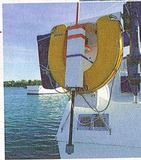
ABOVE Pull the red dowel to release the dan buoy LEFT Dan buoy float is ply and polystyrene
