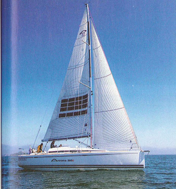
Sails with solar panels sewn in are an emerging technology
