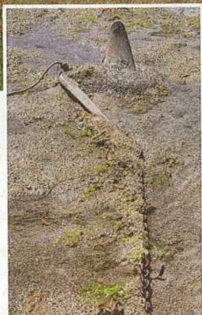
A hinged-plough blade digs itself into the sea bed with its edge before rotating its point downwards
