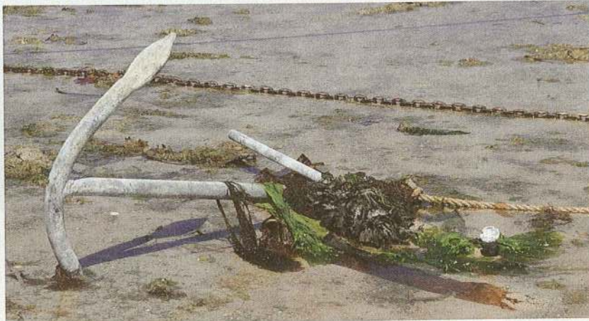
The Fisherman anchor sticks one fluke in like a spear, but it is only a small spear
