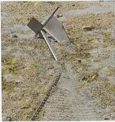
A Danforth-type anchor may turn over if the cable swings to one side and makes it rotate about its stabilising bar
