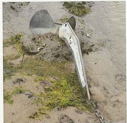
In thin sand over hard clay, this Delta was unable to dig in but dragged slowly until its point lodged in a clay crevice
