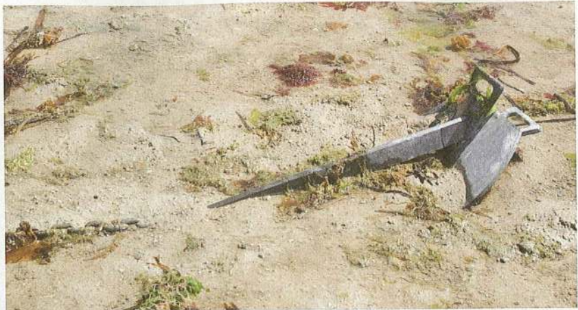
Britany anchors, and derivatives such as this FOB, are fairly tolerant of thin weed, but may corkscrew under very high loads
