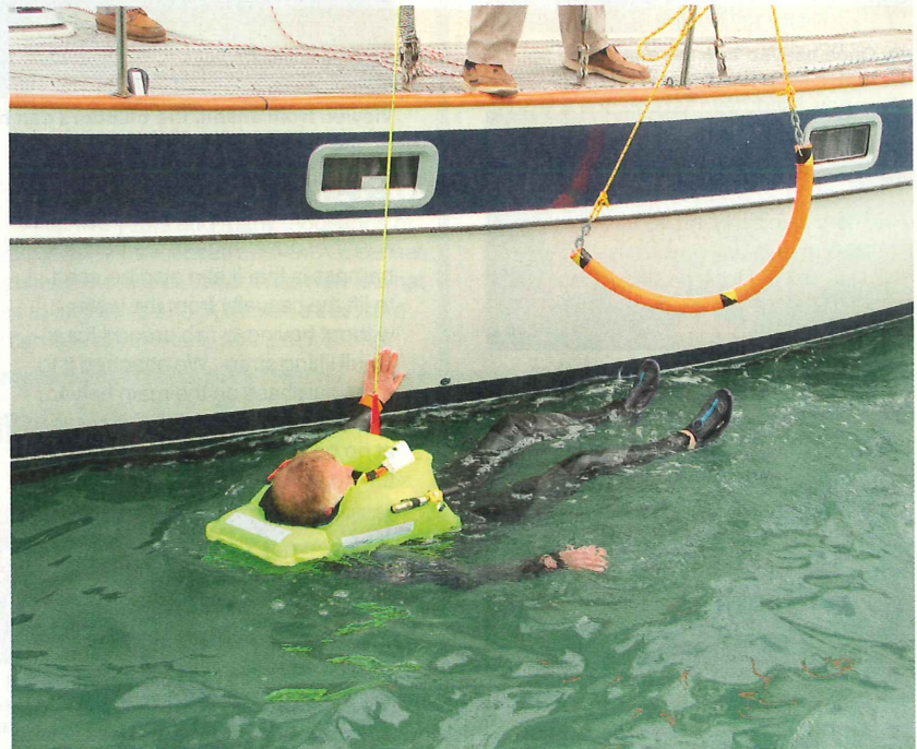
5 Duncan's solution is to use a piece of chain encapsulated in plastic pipe, with a rope strop. This he lowers into the water.
