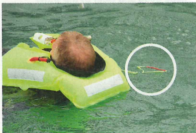
1 Tony, our victim, falls in. As the lifejacket inflates, the floating Dyneema line is propelled free and floats nearby.
