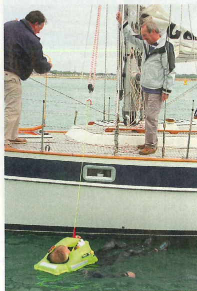
4 You can lift the casualty like this – but he runs the risk of hydrostatic squeeze, whereby as he exits the water vertically, the squeeze of the water pressure on the legs reduces and the blood rushes to his feet, dropping blood pressure – which can strain the heart.
