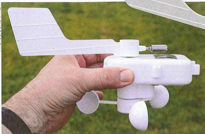
The small masthead unit is solar powered and requires no wiring
