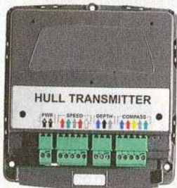
LEFT Speed, depth and compass transducers are wired to the powered Hull Transmitter, which then distributes the data wirelessly
