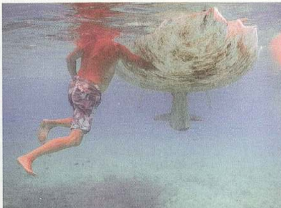
Andrew cleaning Nightstar's bow thruster and hull
