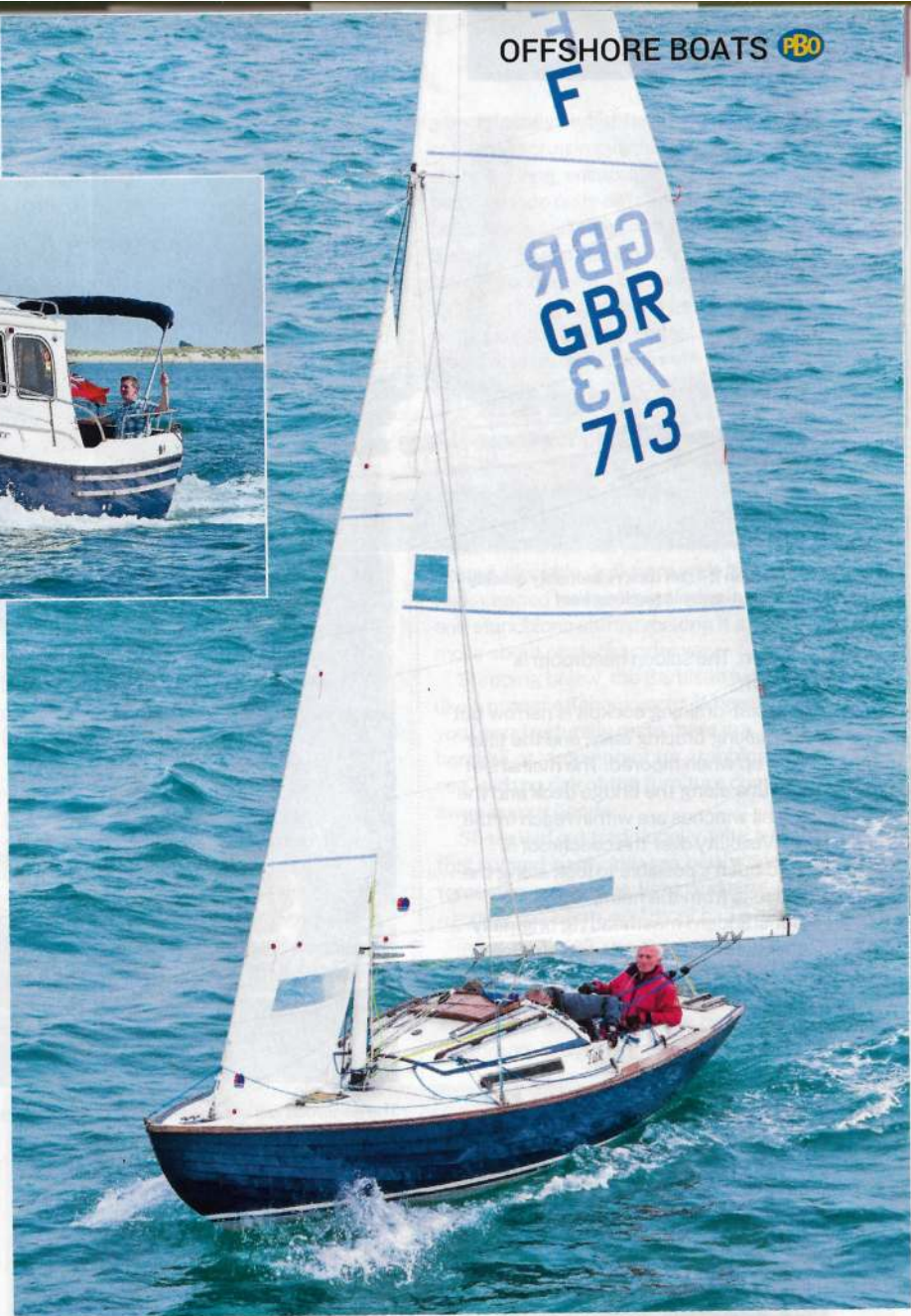
Small headsails make the rig of the Folkboat easy to handle. The boat is also stiff and well balanced
