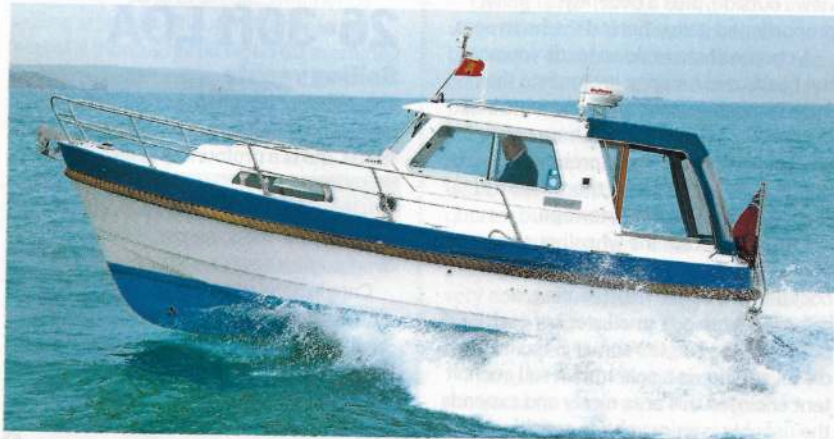
The modern planing underbody on the Hardy Mariner 26 delivers around 22 knots
