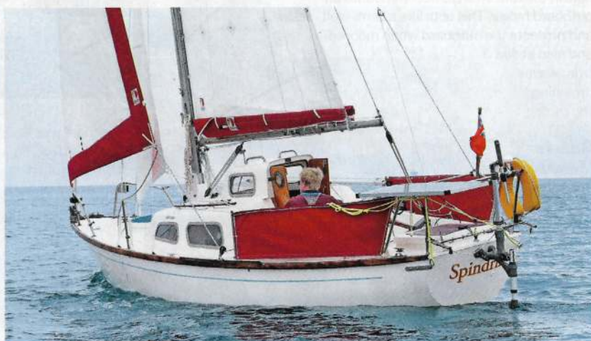
A large proportion of the Hurley 22s sold had twin keels, drawing 2ft 6in
