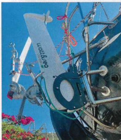
The Watt & Sea hydrogenerator worked well as long as the boat speed was 4 knots or more
