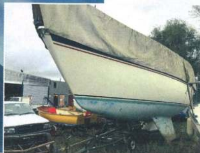
BELOW A well fitted full deck cover can protect a yacht from the elements for several years
