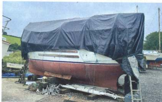
RIGHT a full cover using hoops, allowing for a full rebuild inside – highly effective, has lasted over 12 months
