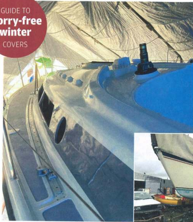
LEFT Scaffold tent with light cover – worked well for a respray as the light was great, but is sadly not robust enough to cope with winter winds
