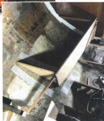
This bunk-front is glassed-in when warm but the rest of the bunk can be built later
