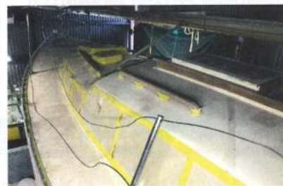
The superstructure must be faired and painted before the weather turns
