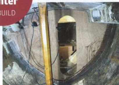
Extensive fibreglass work, like glassing in large bulkheads, is warm weather work
