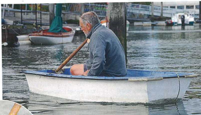
Here's an example of a pram tender being sculled while the skipper is sitting down. INSET LEFT A thick leather lining to the sculling notch keeps noise down and prevents wear to the oar
