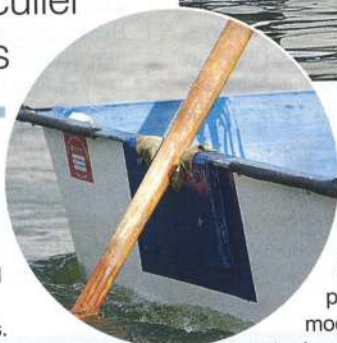
Here's an example of a pram tender being sculled while the skipper is sitting down. INSET LEFT A thick leather lining to the sculling notch keeps noise down and prevents wear to the oar
