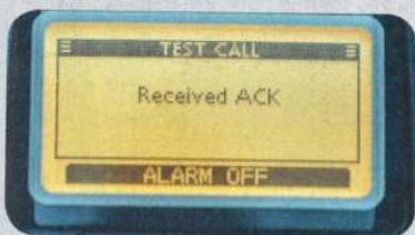
The ICOM sounds an alarm and says it has received the acknowledgement. Cancelling the alarm moves it on to the next screen.
