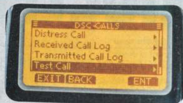
'Test call' selected in the DSC menu. Note 'Distress Call' is three above: DO NOT select this.
