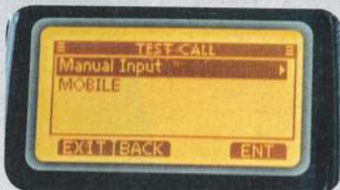
Here I have to select station to call. Either I put in a new station by selecting 'Manual' or select one from the directory. In my case I selected 'Mobile' > my Standard Horizon.
