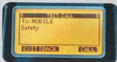
The radio shows me what I have selected and offers me the chance to 'Exit' (go back and perhaps use another number from my directory), or 'Call' (send the message).
