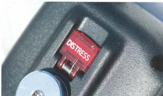
This DSC test procedure does not involve pressing the red button. It is a menu option within the radio itself
