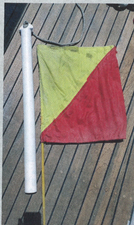
Dan buoy flag cover is tethered to the backstay and held in place by gravity
