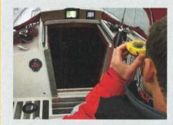
HANDBEARING COMPASS An alternative to this process is to simply compare your hand bearing compass to your steering compass. Stand on the centerline and sight the slot in the mast with your hand bearing compass. Run the boat along a course N, S, E and W and compare the difference to the main compass.
