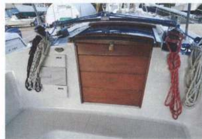
ABOVE Though seakindly, a compact interior can feel claustrophobic at times. ABOVE RIGHT Old boats tend to have companionway washboards rather than the popular hinged doors that make entry a joy on newer yachts
