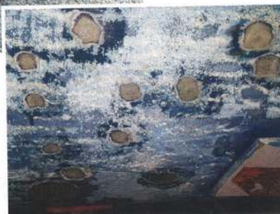
Blisters, blisters, and more blisters on this well-maintained boat demonstrate the unrelenting marine environment
