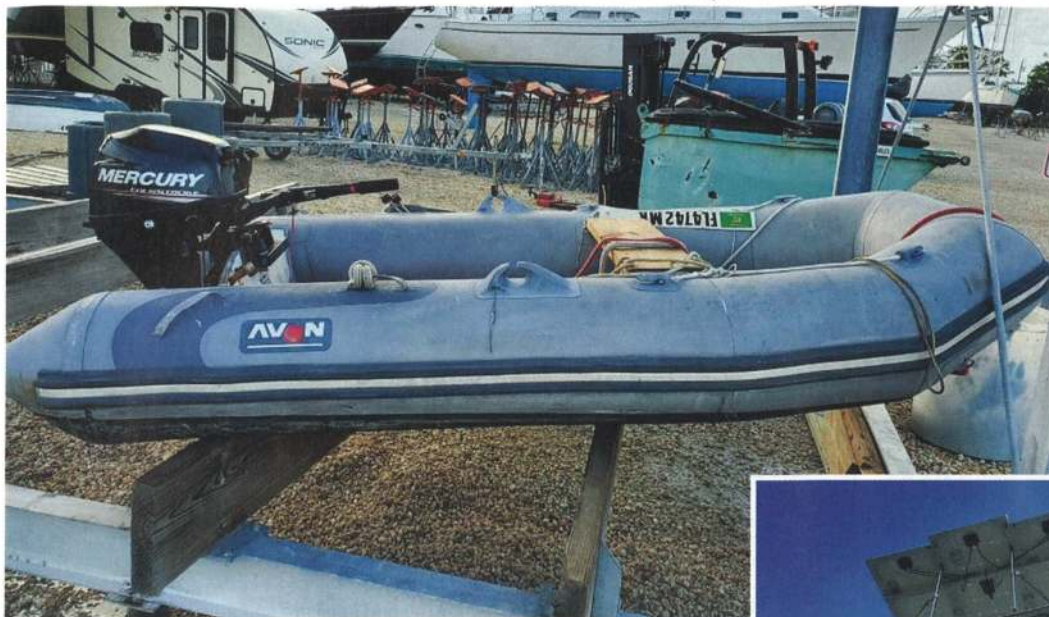
LEFT A good dinghy is a great investment. Our hypalon Avon dinghy will do about 17 knots with its 9.9hp outboard and is a good platform for fishing, diving, and exploring rivers and beaches
