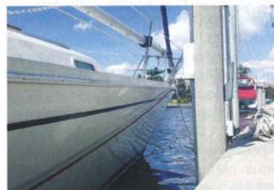
Aged gelcoat requires constant cleaning and polishing to stay looking like this
