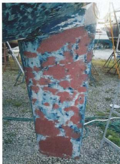
It's prudent to drop rudders on old boats to check the bearings and shaft
