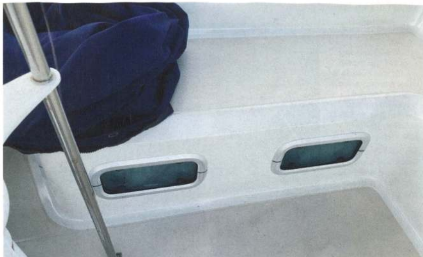
ABOVE LEFT Intense UV over decades crazes and wears out port lenses, seals, and latches. ABOVE RIGHT Old boats feature beautiful and teak interiors, but also annoying Formica countertops. In my view, Corian is much preferred
