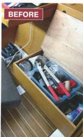
Bolt cutters were stowed in a locker in the saloon – too far from the deck where they'll be needed
