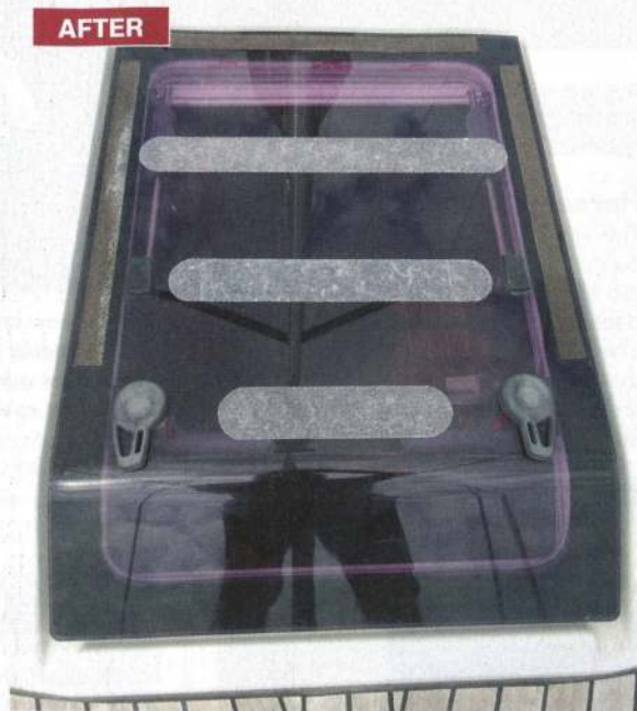
LEFT Hatch over the companionway is regularly used when stowing the mainsail, so it got the non-slip treatment
