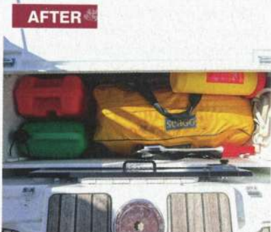
We eventually had to stow the dinghy fuel tanks in with the liferaft as the other cockpit locker wasn't fitted with drains
