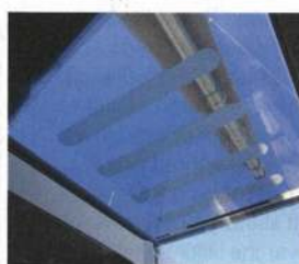
LEFT Hatch over the companionway is regularly used when stowing the mainsail, so it got the non-slip treatment
