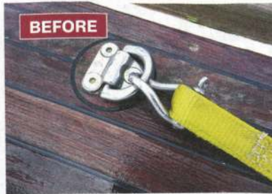
ABOVE Jackstays were fitted and in good condition but the shackles were not wired... that was simply remedied (right) with plastic cable ties
