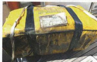
The liferaft was situated in this admirably uncluttered lazarette locker, but the drain was blocked so the raft was sitting in water and was out of date, so we sent it for servicing. The locker lid also needed attention so it could be fully removed to extract the liferaft
