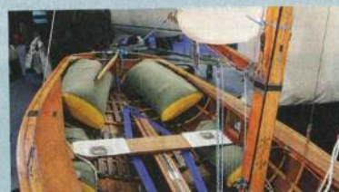
10 Add buoyancy using builder's foam in a dry-bag: p84, April 2018.
