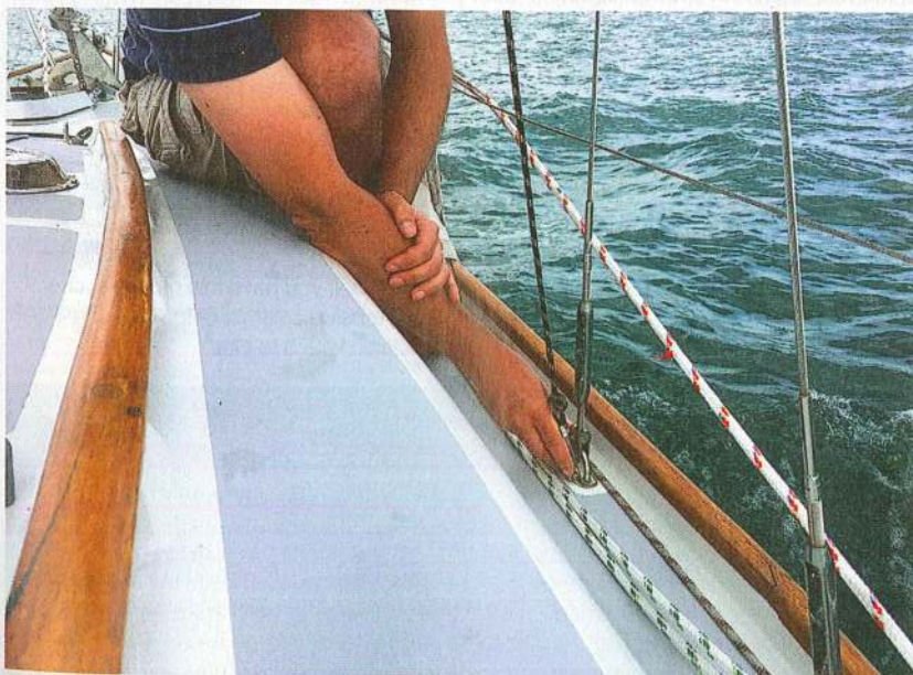
Use the main halyard to measure to the cap shroud chainplates on both sides
