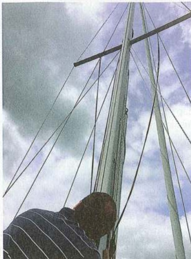
Sight up the luff groove to check that the mast is in column from side to side
