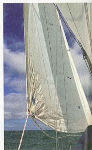
In a moderate breeze the leeward shrouds should stay taut
