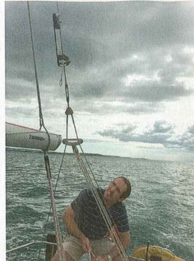
With a backstay bridle like this, check the tension above the joining plate
