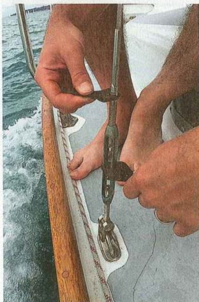
Use a second spanner to hold the shroud still when tensioning the bottlescrew
