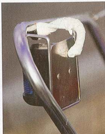
Protecting vulnerable wires could increase their working lifespan
