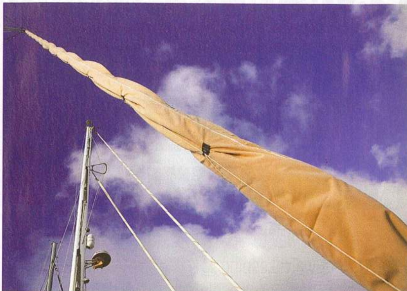
Replacing a sock every few years is much cheaper than replacing a sail
