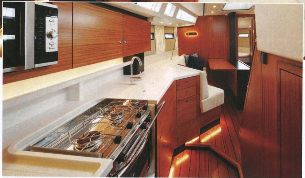
The galley is over 2m (6ft 7in) long and is well designed for use at sea. Some fiddles outboard would give extra storage space for smaller items. The Corian top from the galley goes all the way to the forward bulkhead
