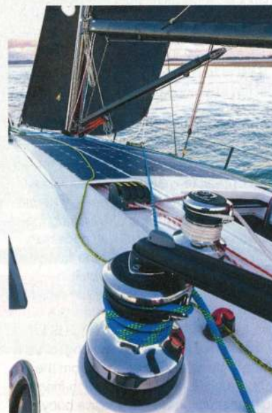
Cross-wincing means you can sheet in and trim the headsail from the windward side using the Seldén reversible winches. The solar panel can be walked on
