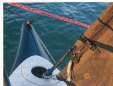
Set on a torsion rope , the jib is designed to be furled rather than reefed. The drum is below the deck
