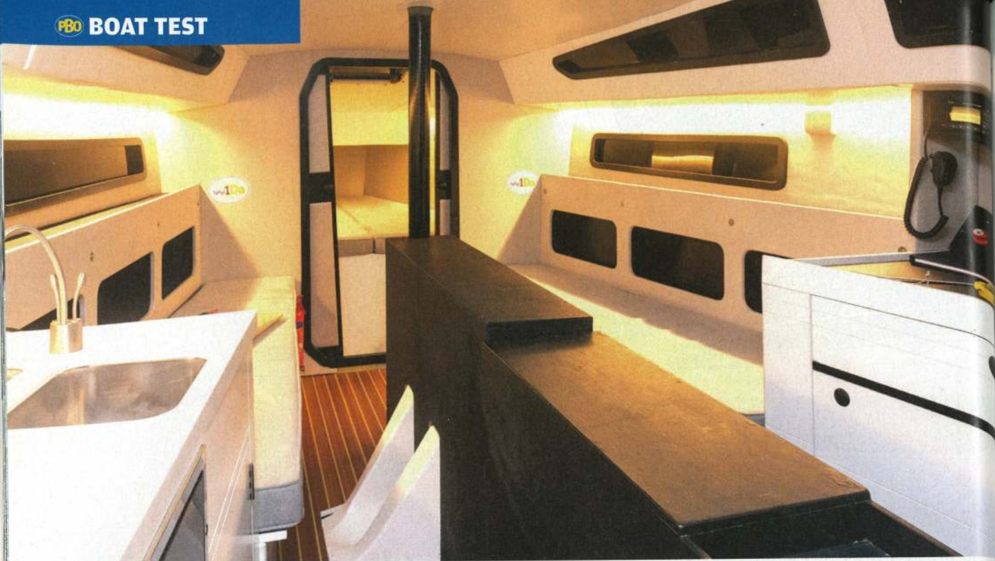
ABOVE The keel case inevitably dominates the saloon, but provides a useful bracing point for working at the chart table or galley
