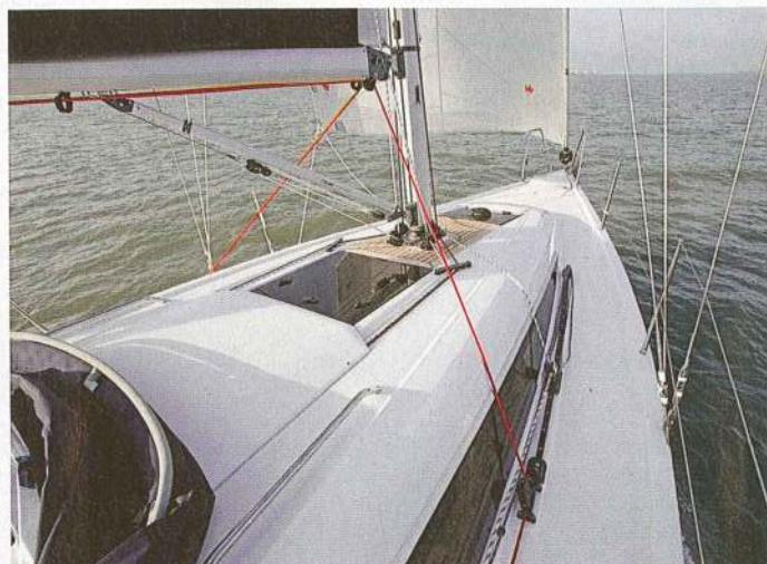
The mainsheet may be a trip hazard for crew standing on the cabin top
